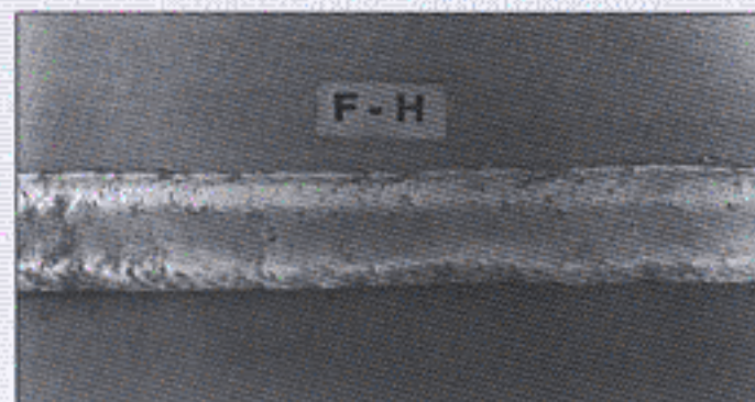
Horizontal fillet welding: 250 amp
